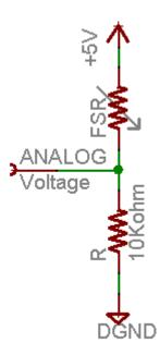
For this example I'm showing it with a 5V supply but note that you can use this with a 3.3v supply just as easily. In this configuration the analog voltage reading ranges from 0V (ground) to about 5V (or about the same as the power supply voltage).
