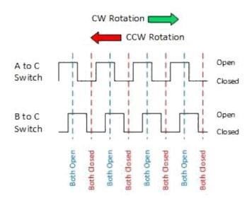
Essentially, determining which switch changed states rst is how the direction of rotation is determined.
