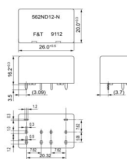
• PC board mounting hole layout (BOTTOM VIEW)
